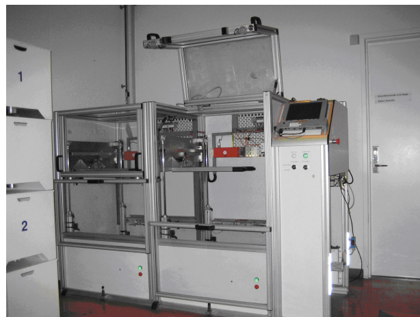
Fig. 5. Minimal station configuration; two loading/unloading cells and human interface.
